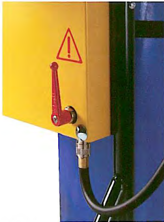
Emergency Relief Valve
